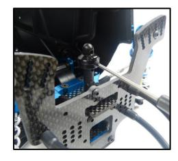
13. Position the tail tank on the body post and install the body clip.
