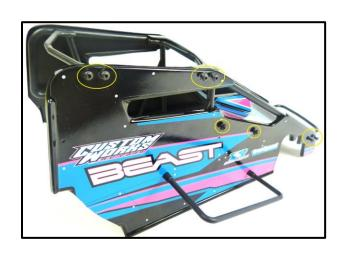
10. Locate the 8pcs of 5348 M3x8 Flat Head screws and use them to fasten the cage assembly to the chassis as shown.
