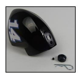
12. Install the set screw into the body post collar and snug the set screw into place on the body post in the position shown. Be careful not to overtighten the set screw.
