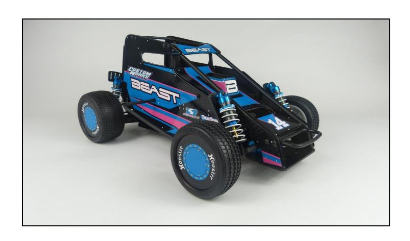
Basic set-up — use the included turnbuckle wrench to fine tune the steering and camber links. Begin with a slight amount of toe-out on the front wheels. Make sure the servo saver is centered when the wheels are centered. Adjust the camber links so that the top of all 4 tires lean to the left slightly (1 degree.)
