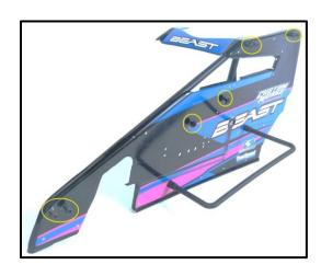
5. Install the halo bars and front bumper with the steel screws. Mount the left side of the hood using the nylon screws & nuts.
