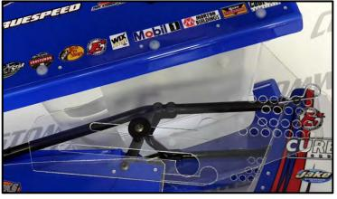
7. Front wing – Assemble the front wing and mount to the front nerf bar as shown.
