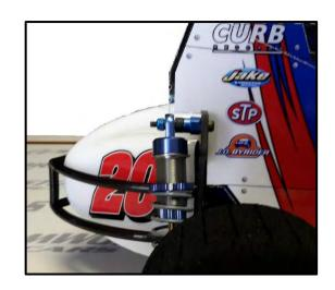
4. Headers – trim headers and drill (2) .125 mounting holes on each. Mount as shown using the inner header holes in the side panels.
