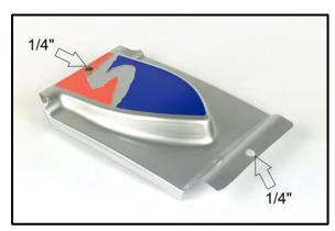
2. Nose piece – Cut along the trim lines as shown and drill 1/8" holes on the (6) dimples for the front nerf bar mount.
