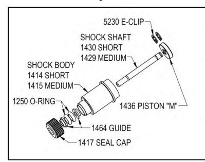
ASSEMBLE 2 SHORT SHOCKS FOR FRONT OF CAR AND 2 MEDIUM SHOCKS FOR REAR OF CAR.
