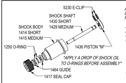
ASSEMBLE 2 SHORT SHOCKS FOR FRONT OF CAR AND 2 MEDIUM SHOCKS FOR REAR OF CAR.
